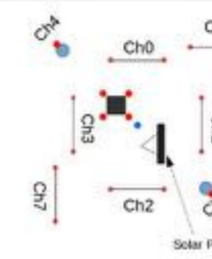
Ch0 - 3: downward facing LPDA Ch5 & 7: upward facing LPDA Ch4 & 6: dipole antennas
